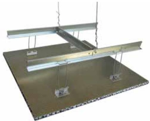
CMP torsion spring **accessible** system with 1<sup>3/8</sup>" grid
