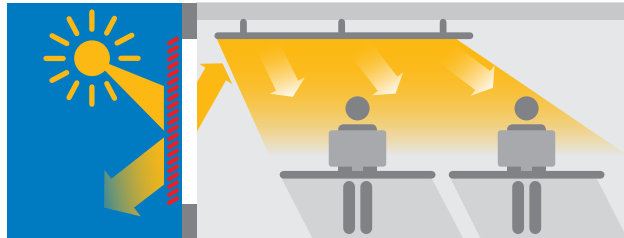
Daylight deflection into the heart of rooms using Atlantic with active solar protection
